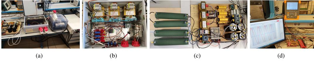
Fig. 4. Test bench: (a) VSI and  $LC$  filter, (b)  $LC$  filter and voltage and current sensors, (c) non-linear load and, (d) control hardware and user interface.
