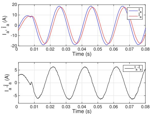
Fig. 11. Performance of the FCS-MPC controller with observer proposed in [13] and  $J_{gain} = 1e4$  under load step. Top: Output current and estimate for phase  $a$ . Bottom: Difference between actual and estimated current for phase  $a$ .
