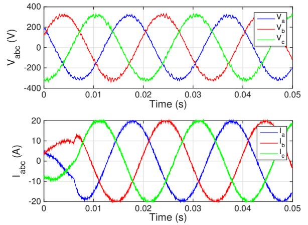
Fig. 12. Performance of the FCS-MPC controller with the new proposed observer and  $J_{gain} = 1e4$  under load step. Top: Output voltages. Bottom: Output currents.
