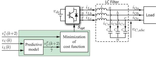
Fig. 2. Block diagram of the FCS-MPC applied to the VSI with output LC filter.
