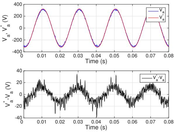
Fig. 4. Performance of the FCS-MPC controller with observer proposed in [13] and  $J_{gain} = 1e4$ . Top: Output voltage and reference for phase  $a$ . Bottom: Tracking error for phase  $a$ .
