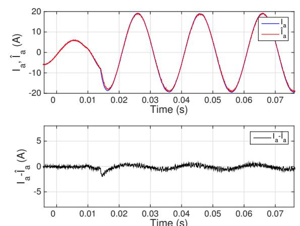
Fig. 14. Performance of the FCS-MPC controller with the new proposed observer and  $J_{gain} = 1e4$  under load step. Top: Output current and estimate for phase  $a$ . Bottom: Difference between actual and estimated current for phase  $a$ .
