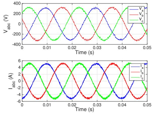
Fig. 6. Performance of the FCS-MPC controller with the new proposed observer and  $J_{gain} = 1e4$ . Top: Output voltages. Bottom: Output currents.
