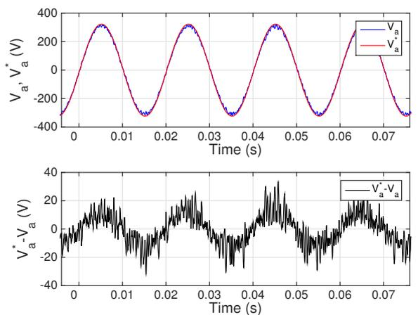
Fig. 13. Performance of the FCS-MPC controller with the new proposed observer and  $J_{gain} = 1e4$  under load step. Top: Output voltage and reference for phase  $a$ . Bottom: Tracking error for phase  $a$ .
