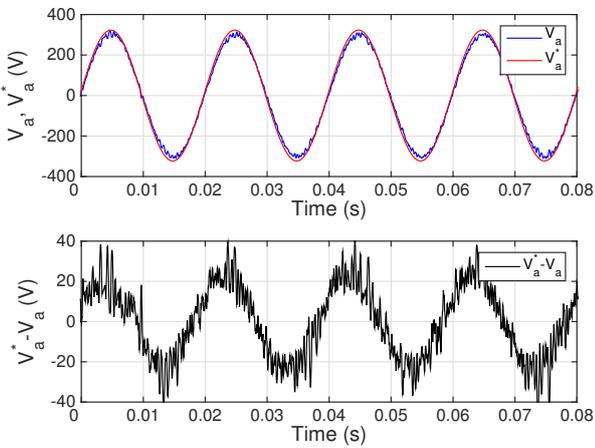
Fig. 10. Performance of the FCS-MPC controller with observer proposed in [13] and  $J_{gain} = 1e4$  under load step. Top: Output voltage and reference for phase  $a$ . Bottom: Tracking error for phase  $a$ .
