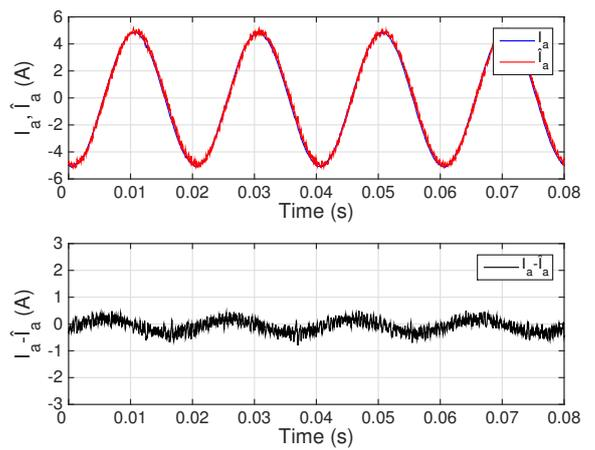
Fig. 8. Performance of the FCS-MPC controller with the new proposed observer and  $J_{gain} = 1e4$ . Top: Output current and estimate for phase  $a$ . Bottom: Difference between actual and estimated current for phase  $a$ .
