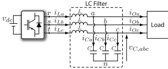
Fig. 1. Scheme of the inverter connected to the output LC filter and load.
