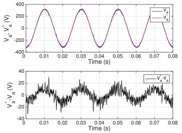
Fig. 7. Performance of the FCS-MPC controller with the new proposed observer and  $J_{gain} = 1e4$ . Top: Output voltage and reference for phase  $a$ . Bottom: Tracking error for phase  $a$ .
