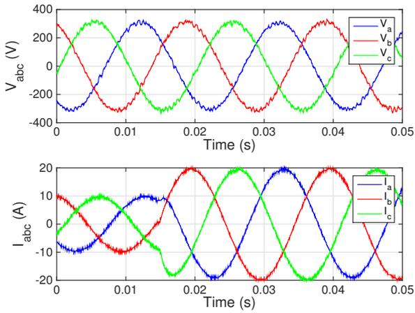
Fig. 9. Performance of the FCS-MPC controller with observer proposed in [13] and  $J_{gain} = 1e4$  under load step. Top: Output voltages. Bottom: Output currents.
