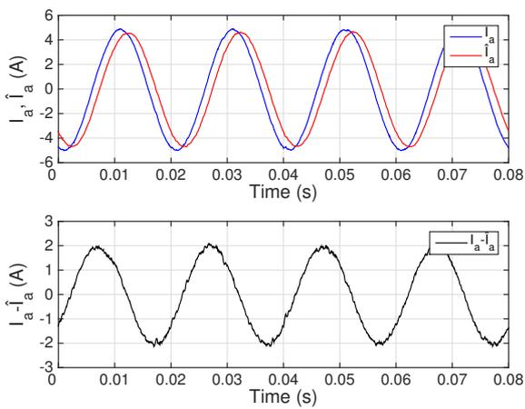
Fig. 5. Performance of the FCS-MPC controller with observer proposed in [13] and  $J_{gain} = 1e4$ . Top: Output current and estimate for phase  $a$ . Bottom: Difference between actual and estimated current for phase  $a$ .
