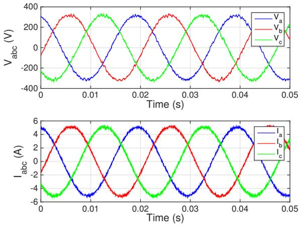
Fig. 3. Performance of the FCS-MPC controller with observer proposed in [13] and  $J_{gain} = 1e4$ . Top: Output voltages. Bottom: Output currents.
