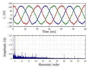
(b) Three-phase stator current waveforms and harmonic spectrum; the rms amplitude of the phase current is 85 A. MP<sup>3</sup>C produces 3.77% total demand distortion (TDD) referred to the rated current of the controlled machine (137 A).
