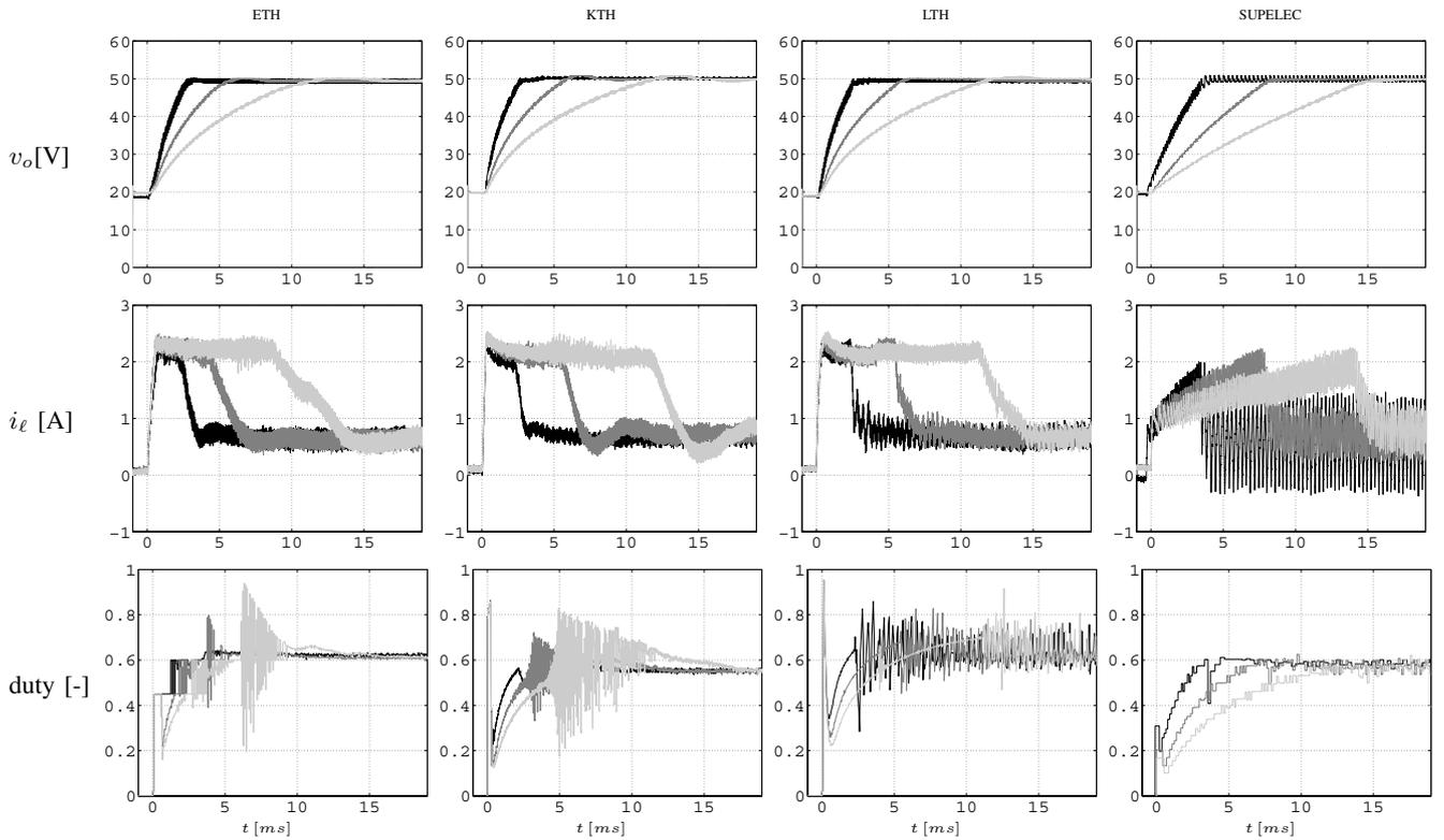
Fig. 15. Boost converter: robustness evaluation. Start-up transient for three different values of capacitor:  $x_c = 50F, 100F, 200F$ .  $v_s = 20V$ ,  $v_{o,ref} = 50V$ ,  $r_o = 200\Omega$
