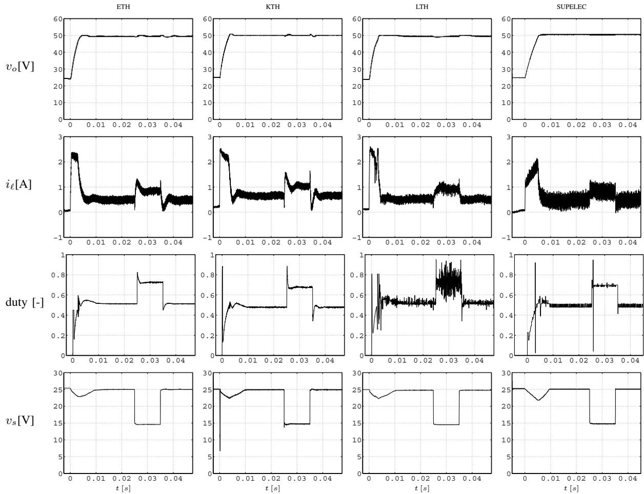
Fig. 16. Boost converter: start-up and line transient. At time  $t = 25$  ms a step-down from  $v_s = 25$  V to 15 V is applied on the supply voltage. At time  $t = 35$  ms a step-up to the initial value is applied.  $v_{o,ref} = 50$  V,  $r_o = 200 \Omega$
