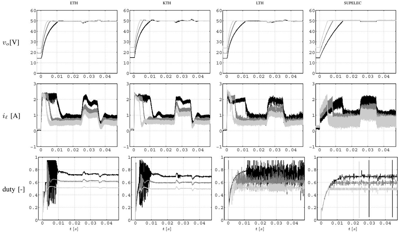
Fig. 14. Boost converter: start-up and load transient. At time  $t = 25$  ms, a load step from  $200 \Omega$  to  $100 \Omega$  is applied. At time  $t = 35$  ms a step back to the initial value is applied.  $v_s = 15V, 20V, 25V$ ,  $v_{o,ref} = 50V$ .
