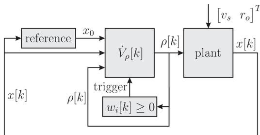
Fig. 8. Discrete-time implementation of SUPELEC control scheme. Control input is evaluated when block  $w_i \geq 0$  triggers the control law. Reference block adjust reference trajectory for robustness to disturbance and improved transient performance.
