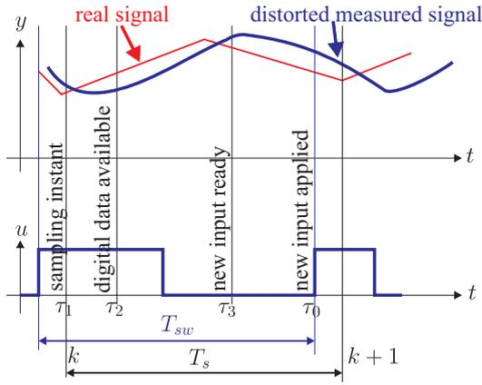
Fig. 9. Time diagram of the control process events.
