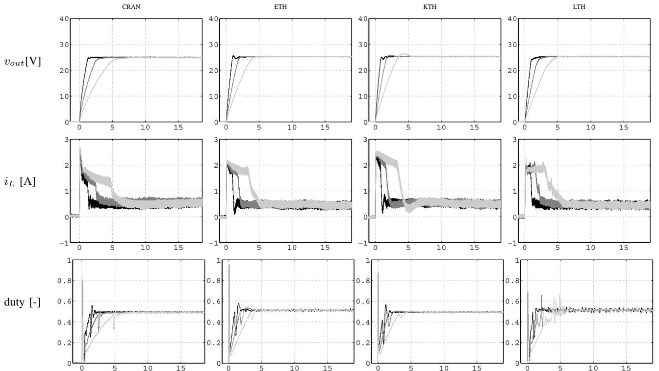
Fig. 11. Buck converter; start-up transient for three different values of the capacitance  $x_c$  (Robustness evaluation). The values are  $x_c = 0.5x_{c,nom}$  (black),  $x_c = x_{c,nom}$  (gray) and  $x_c = 2x_{c,nom}$  (light gray) where  $x_{c,nom} = 100\mu\text{F}$  is the nominal value.  $v_s = 50\text{V}$ ,  $v_{o,ref} = 25\text{V}$ ,  $r_o = 50\Omega$ . The group results are presented side by side.
