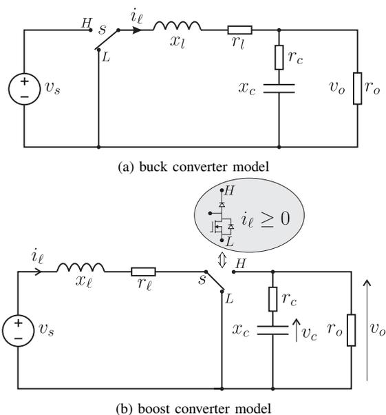
Fig. 2. Lumped parameter circuit used for control synthesis
