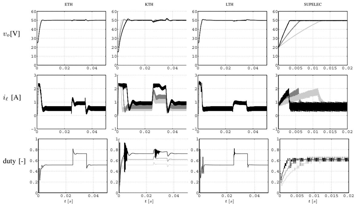
Fig. 17. Boost converter: selected simulation results for comparison with experiments.
