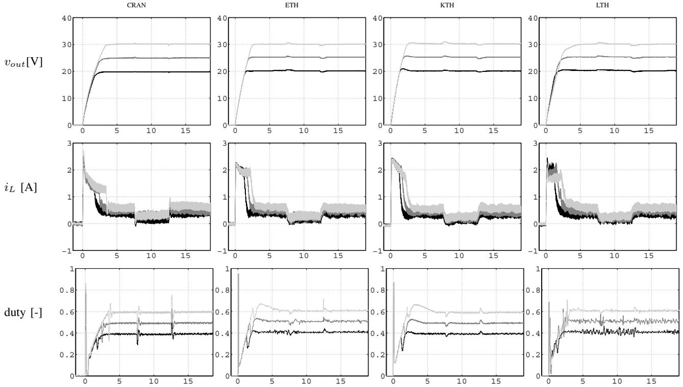
Fig. 10. Buck converter; start-up transient and response to a step in the load resistance from  $r_o = 50\Omega$  to  $r_o = 100\Omega$  and back again. The experiment is performed for three different values of the reference output voltage  $v_{o,ref}$ . The values are 20V (black), 25V (gray) and 30V (light gray). The experiments of the four groups are presented side by side.
