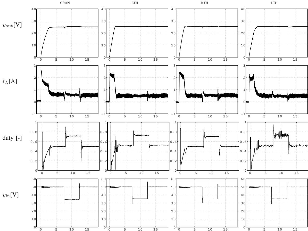
Fig. 12. Buck converter; start-up transient and response to a step in the source voltage from  $v_s = 50\text{V}$  to  $v_s = 35\text{V}$  and back again.  $v_{o,\text{ref}} = 25\text{V}$ ,  $r_o = 50\Omega$ .
