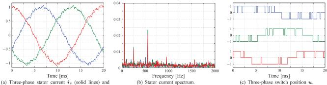
(a) Three-phase stator current  $i_s$  (solid lines) are their references (dash-dotted lines).
