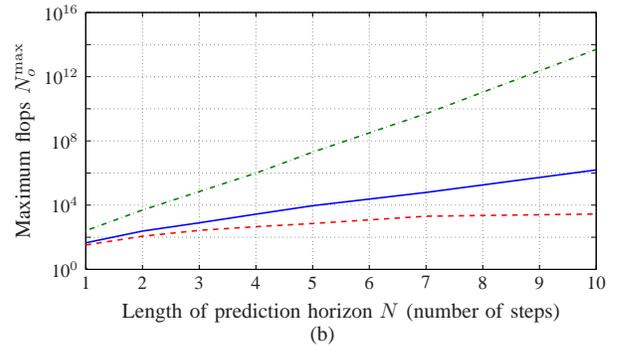
Fig. 6: Maximum number of flops  $N_o^{max}$  performed during the search process when the (a) step-down and (b) step-up torque reference changes in Fig. 5 occur as a function of the prediction horizon  $N$ . The solid (blue) line refers to the sphere decoder in [3], the dashed (red) line to the presented algorithm, and the dash-dotted (green) line to the exhaustive enumeration.
