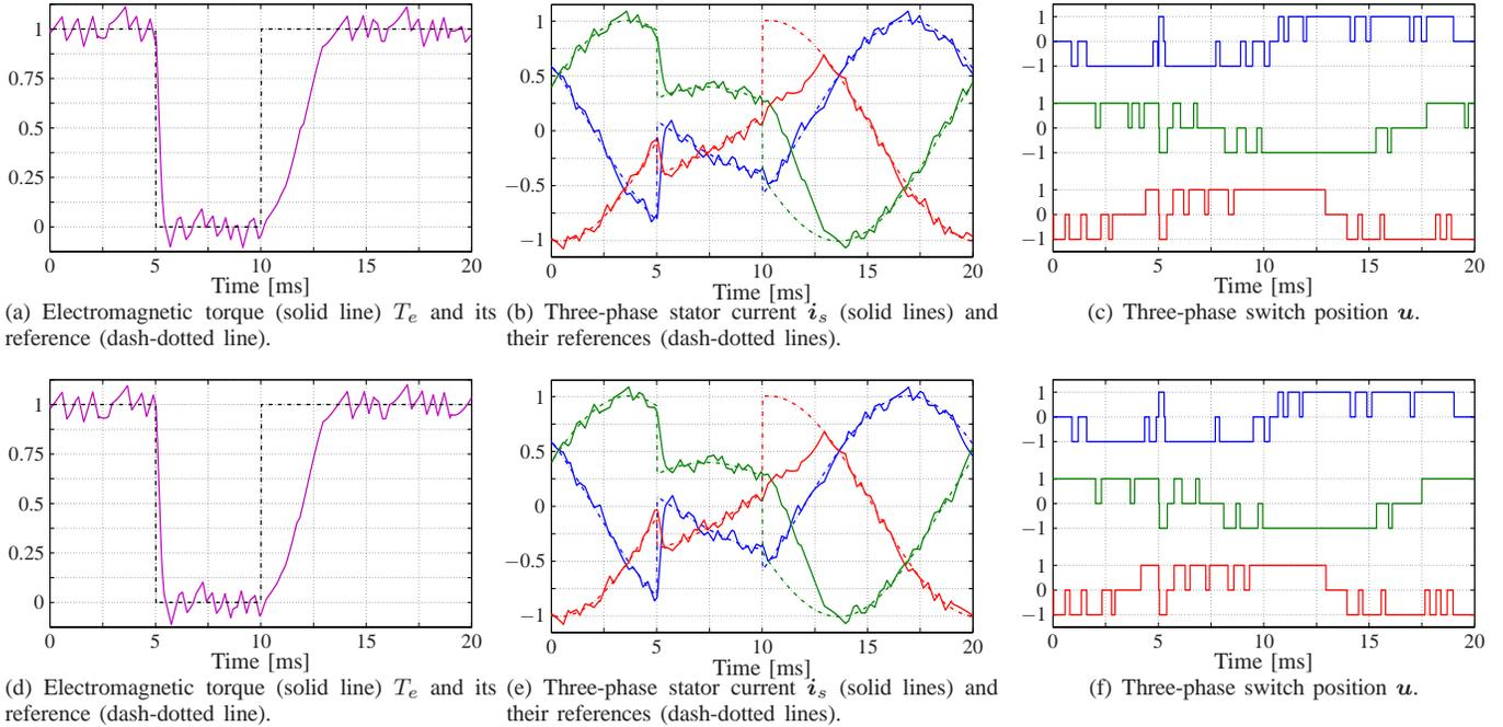
Fig. 5: Torque reference steps for direct MPC with a ten-step horizon ( $N = 10$ ) at nominal speed. The sampling interval is  $T_s = 25 \mu\text{s}$  and the switching frequency is approximately 300 Hz ( $\lambda_u = 0.1$ ). (Upper row) Simulated waveforms with the original sphere decoder (see [3]). (Lower row) Simulated waveforms with the modified sphere decoder (i.e., the proposed approach).
