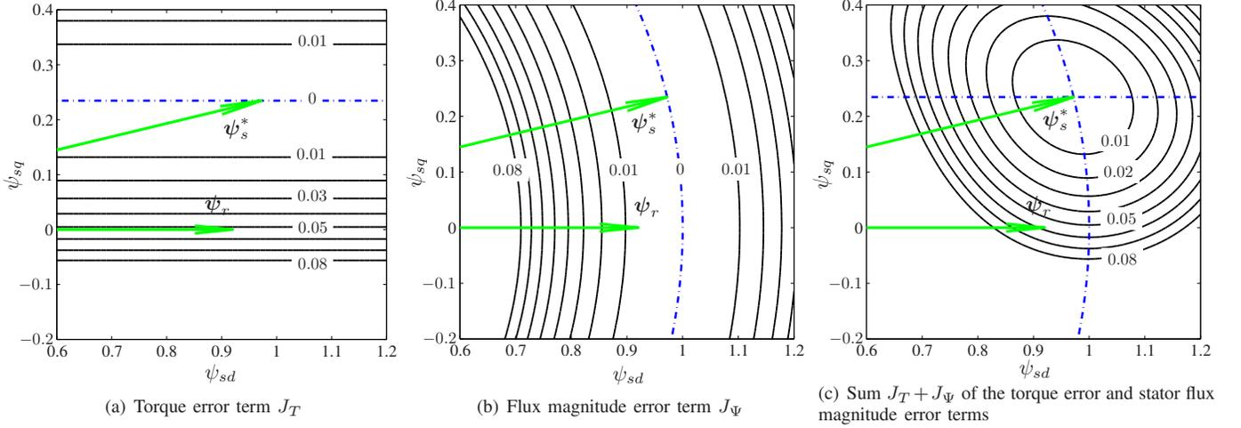
Fig. 3: Contour maps of the cost function terms of the predictive torque and flux controller in a plane spanned by the  $d$ - and  $q$ -components of the stator flux vector. The reference stator flux and the rotor flux vectors are shown as arrows
