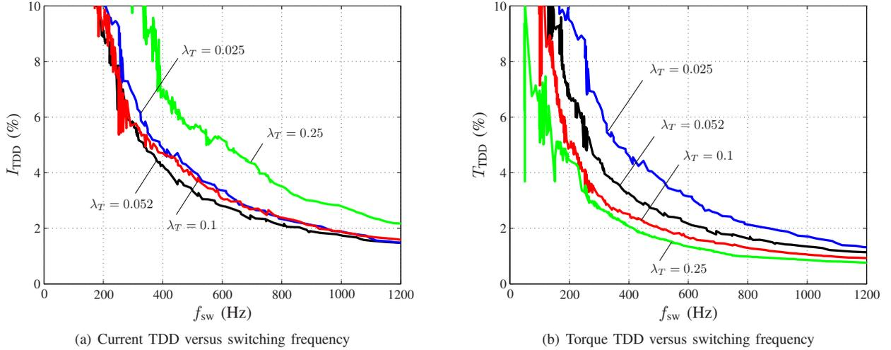
Fig. 9: Predictive torque and flux control with different torque weights  $\lambda_T$  when operating at nominal speed and rated torque
