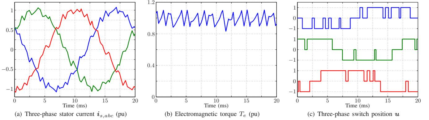
Fig. 7: Predictive torque and flux control during steady-state operation for  $\lambda_T = 0.052$  and  $\lambda_{uT} = 0.198 \cdot 10^{-3}$ , with  $I_{TDD} = 7.74\%$  and  $f_{sw} = 221$  Hz
