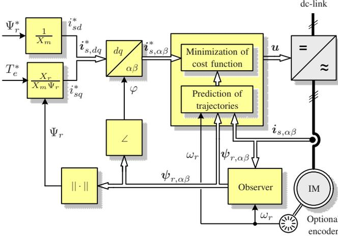
Fig. 4: Block diagram of the predictive current controller
