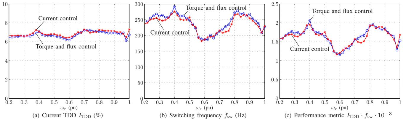
Fig. 11: Predictive torque and flux control versus predictive current control. Operation at zero torque ( $T_e^* = 0$  pu) and multiple speed operating points  $\omega_r$ .
