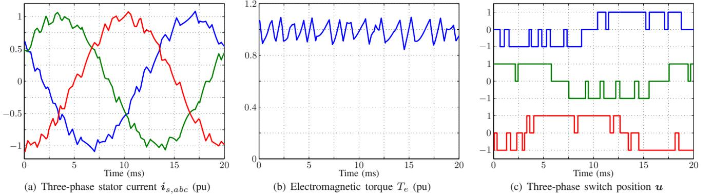
Fig. 8: Predictive current control during steady-state operation for  $\lambda_{uI} = 3 \cdot 10^{-3}$ , with  $I_{TDD} = 6.69\%$  and  $f_{sw} = 222$  Hz
