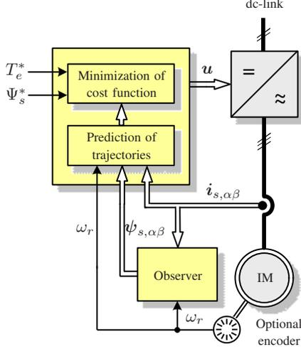
Fig. 2: Block diagram of the predictive torque and flux controller
