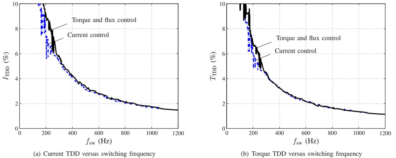
Fig. 10: Predictive torque and flux control with  $\lambda_T = 0.052$  is compared with predictive current control when operating at nominal speed and rated torque
