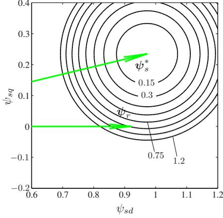
Fig. 5: Contour map of the current error term  $J_I$  of the predictive current controller
