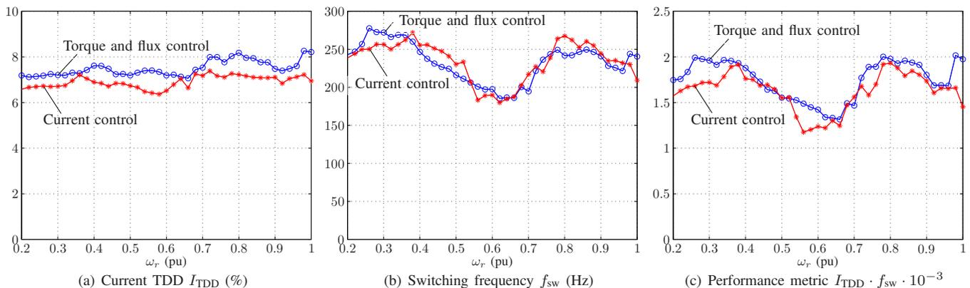
Fig. 12: Predictive torque and flux control versus predictive current control. Operation at rated torque ( $T_e^* = 1$  pu) and multiple speed operating points  $\omega_r$ .
