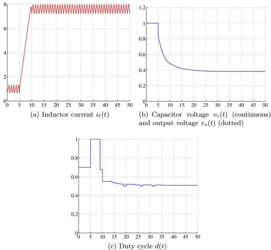
**Fig. 6.** Response of the converter to a step change in the load resistance from  $r_o = 1$  p.u. to  $r_o = 0.05$  p.u. at time-instant  $k = 4$
