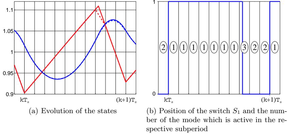
**Fig. 2.** The  $N$ -step modelling approach visualized for the  $k$ -th period. The evolution of the states of the continuous-time nonlinear model (solid lines) is compared with the sequence of states of the discrete-time hybrid model (dashed lines) using  $N = 10$  subperiods, where the saw tooth shaped line represents  $i_l$  and the smooth curve is  $v_c$ .
