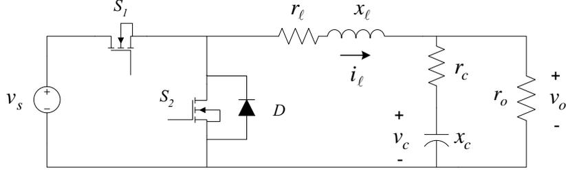
**Fig. 1.** Topology of the step-down synchronous converter
