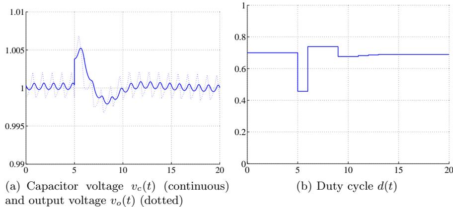
**Fig. 5.** Response of the converter to a step change in the load resistance from  $r_o = 1$  p.u. to  $r_o = 1.5$  p.u. at time-instant  $k = 4$
