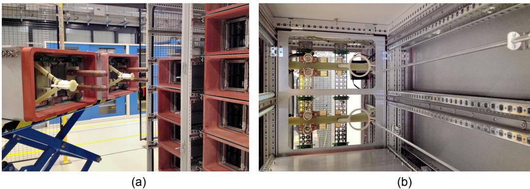
Figure 10: Two PEBBs (a) and cabinets slots for two PEBBs with connecting elements (b).
