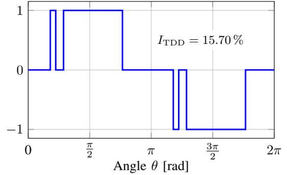
Fig. 6: Half-wave symmetric OPP with  $d = 2$ ,  $m = 0.92$  (corresponding to the cross).
