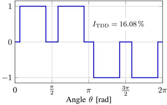
Fig. 5: Quarter- and half-wave symmetric OPP with  $d = 2$ ,  $m = 0.92$  (corresponding to the circle).
