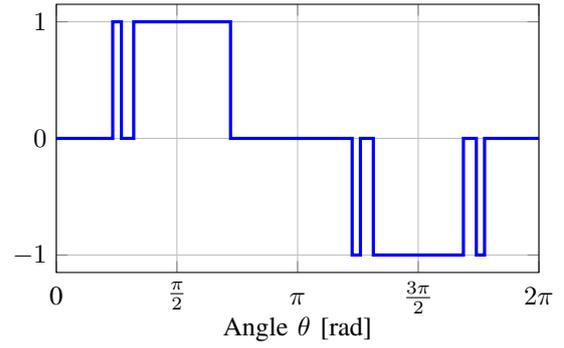
Fig. 10: Full-wave symmetric OPP with  $d = 2.5$  and  $m = 0.9$ .
