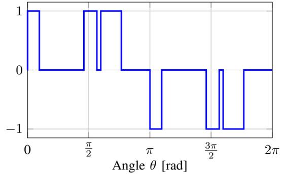
Fig. 8: Half-wave symmetric OPP with  $d = 3$  and  $m = 0.52$ .
