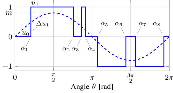
Fig. 1: Single-phase full-wave symmetric pulse pattern (solid line) with  $k = 8$  switching angles  $\alpha_i$  and switching transitions  $\Delta u_i$ . The fundamental component (dashed line) has the amplitude  $\hat{u}_1 = m$ .
