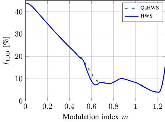
Fig. 7: Current TDDs of quarter- and half-wave (QaHWS) and half-wave symmetric (HWS) OPPs with  $d = 3$ .
