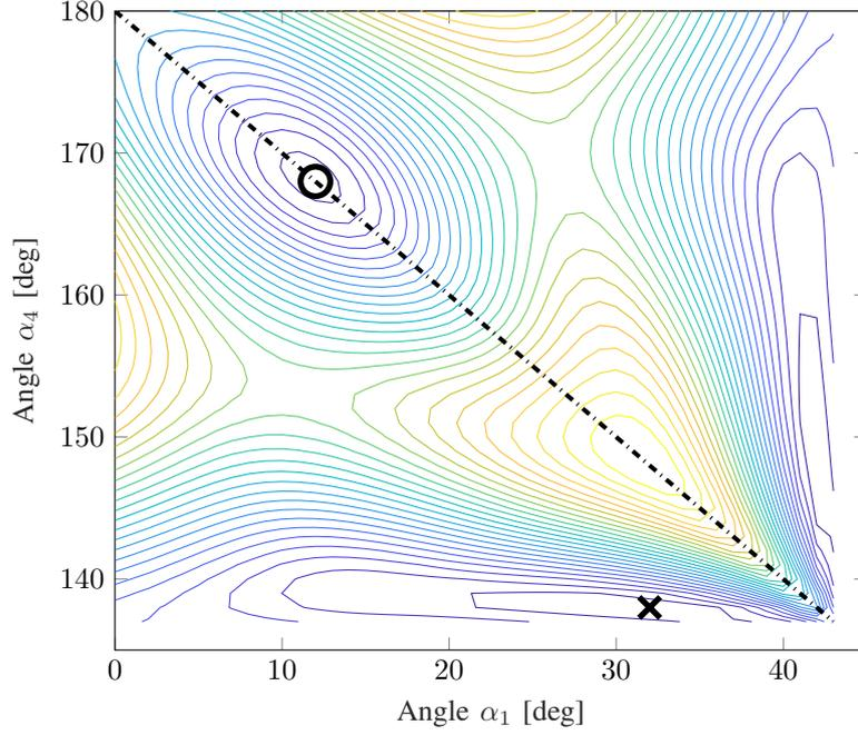
Fig. 4: Cost function in  $\alpha_1$  and  $\alpha_4$  of the half-wave symmetric OPP problem with  $d = 2$ ,  $m = 0.92$ . The cross indicates the half-wave symmetry optimal solution; the circle marks the traditional optimal solution. The dashed line corresponds to the restricted solution space of the traditional problem.
