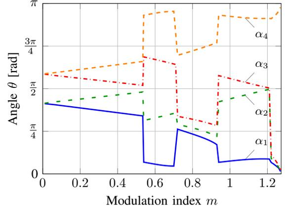
Fig. 3: Switching angles in the first half-wave of the half-wave symmetric OPPs with  $d = 2$
