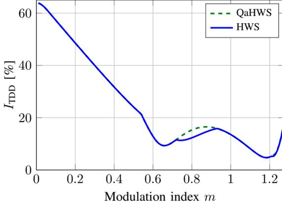
Fig. 2: Current TDDs of quarter- and half-wave symmetric (QaHWS) OPPs and half-wave symmetric (HWS) OPPs with  $d = 2$
